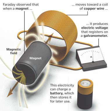
This has made possible the development of the **no-battery flashlight** (also called the **shake flashlight**) which uses motion — provided by the user when he shakes it — to charge an
